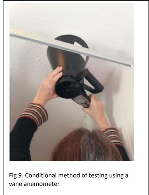
Fig 9. Conditional method of testing using a vane anemometer
