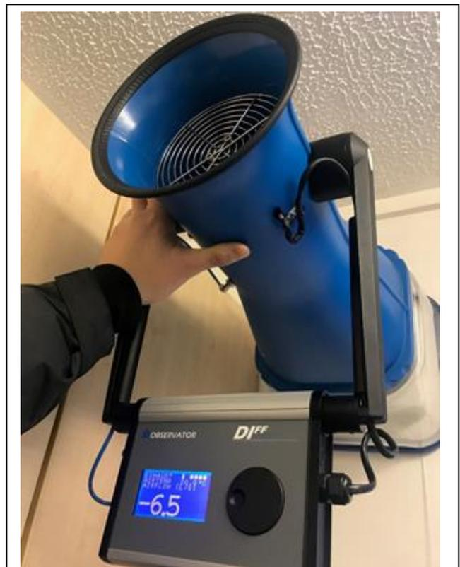
Fig 8. Unconditional method of testing a type 1 ventilation system using a powered hood.
