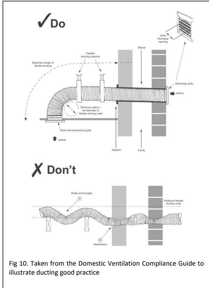
Fig 10. Taken from the Domestic Ventilation Compliance Guide to illustrate ducting good practice
